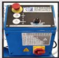
Control Panel with Emergency Stop
