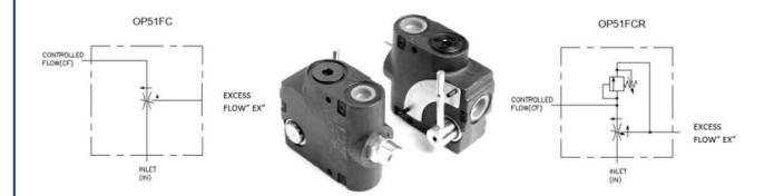
The model OP51FC is a pressure compensated swing arm adjustable flow control valve. By swinging the arm thru 90°, the flow out the CF or controlled flow port can be varied within the range given in the specification.
