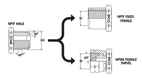
Measure NPT male thread OD and NPT female thread ID at first full thread near end of fitting.
